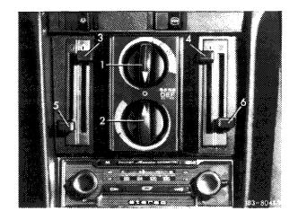
For maximum cooling, temperature vacuum switch (1) is set in range between mark and end of green scale, so that approx. 80 % of recirculated air and approx. 20 % of fresh air are guided through evaporator. Operating levers (12) for heater should be set completely down.
