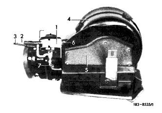
The blower forces the air through the evaporator to the heater box. With the center cooling air outlet (operationg lever 8 at the left) opened the air will flow directly out of center cooling air outlet (4), a slight share of the air is guided through the heat exchangers to the lateral ventilation outlet (3), the defroster nozzles (5) and the rear compartment and legroom openings (6).
