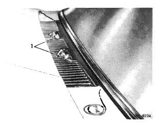
4 Push down bolt on spreader clamps and remove clamps.
