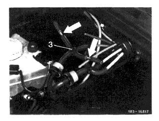
3 Pull check valve (4) out of connection (5).
