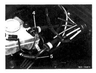
4 Connect tester to check valve (4) (refer to arrow).
