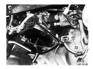
46 Tilt heater box in direction of front wall, while introducing both heater pipes through front wall and into defroster nozzles.
