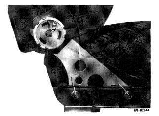
9 Drill out rivets (4) on seat fitting.
