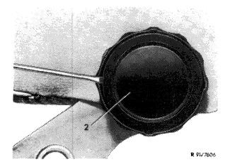
3 Twist spring washer (3) with a screw driver and remove hand wheel.
