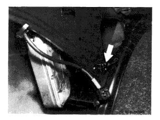
Recesses for speakers are provided on instrument panel left and right.
