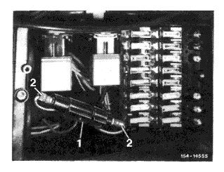
Connections for rear antenna are accessible upon removal of lefthand lining in trunk.
