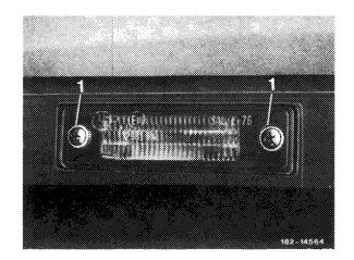
4 Pull cable with coupler inwards after removing rubber grommet (1). Remove righthand and lefthand licence plate lamp from inside.
