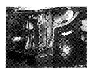
4 Unscrew fastening screws (3). Remove lamp unit and pull off couplers of electrical connections.
