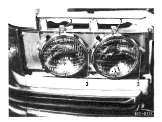
1 Adjusting screw (height)2 Adjusting screw (side)
