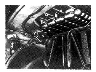
8 Insert partition (60) and attach with hex. screws (61).
