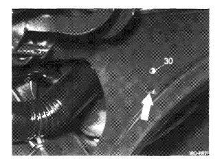
2 Pull vacuum element (4) out of sleeve (19).
