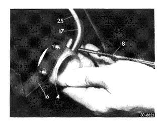
9 Introduce vacuum element (4) into sleeve (19).
