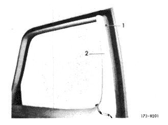
4 Push reveal molding front top (3) out of window frame by means of a plastic wedge.
