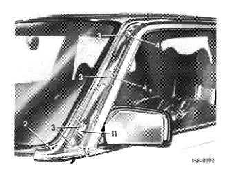
4 Unscrew lateral sheet metal screws (5) and remove ornamental trim (2) in upward direction.
