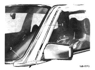
Pull cover (1) out of trimstrip clip (11) in upward direction.
