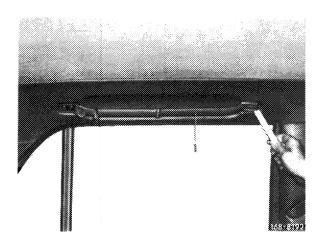
5 Pull lining on roof frame laterally (2) out of reveal molding on windshield top (3) and remove in forward direction.
