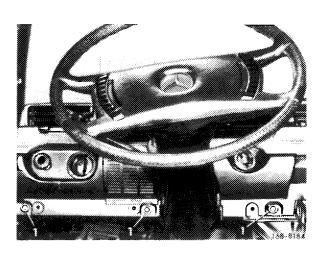
11 Reach through cutout for combination instrument and unscrew nut (2).
