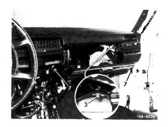
3 Nut (SW 8) right 7 Screws on instrument panel right
