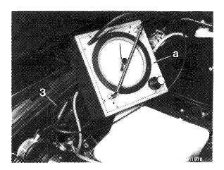
C. Mechanical and pneumatic checkup of actuator, including cable control and control linkage
