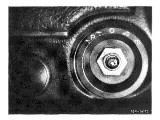
5 Remove lighting switch from instrument panel in downward direction.
