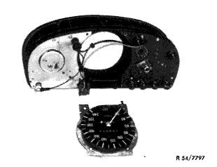
Instrument cluster with time clock and revolution counter
