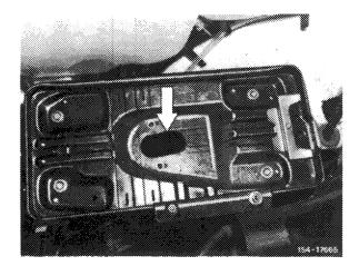
The battery is inclosed in a case which is closed at top by the engine hood.
