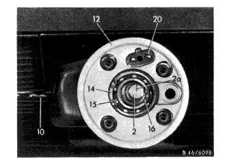
5 On steering wheel 1st version, place spring washer on steering wheel shaft, screw-on hex. nut and tighten to 50 Nm.
