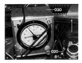
Note: Measuring connection is self-made acc. to specified dimensions (parts 1, 3, 4, 5 and 6 are brazed to each other). For connection to brake unit the pipe fitting including coupling nut of an old vacuum line may be used. Connection to vacuum line is made by means of a screw connection.
