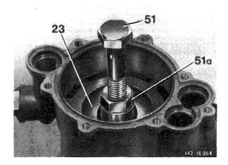
**Note:** The clamping device (51) is self-made acc. to specified dimensions.
