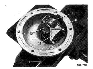
6 Unscrew clamping device (51) from piston rod (17), then remove spring retainer and springs.
