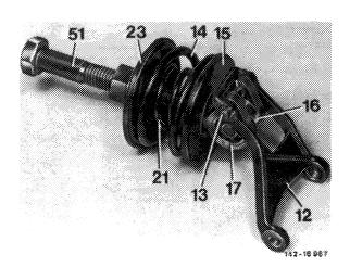
**Note:** Rocker arm with piston rod is available as a complete spare part only. For this reason, disassembly is not required.
