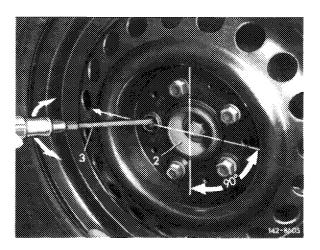
Position of wheel for models with diagonal swing axle and initial torque compensation
