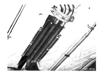
2 Disengage return spring (12) at spring holder (30).
