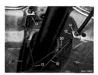
3 Loosen adjusting screw (3) on adjustment bracket (1).
