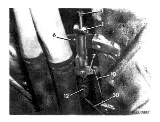
4 Turn steering all the way to left lock and unscrew hexagon nuts (19) in left wheel well.
