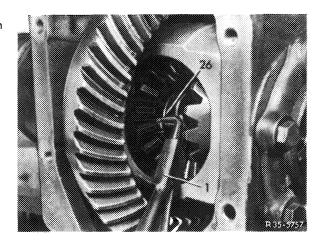
5 Pull rear axle shafts out of side gears and remove together with spacing rings (11).
