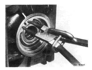
15 Take both bearing outer races of tapered roller bearings (11) from rear axle housing and mark to prevent mixups during reinstallation.
