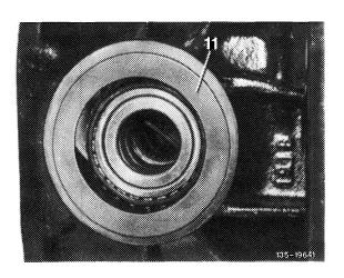
Note: For easier removal of bearing outer races, insert assembly mandrel for differential pinions (046) at the right and force complete differential toward the left until differential rests against rear axle housing. Remove lefthand and righthand bearing outer race.
