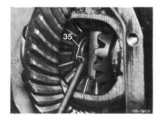
5 Pull rear axle shafts out of differential side gears and remove together with compensating washers (36).
