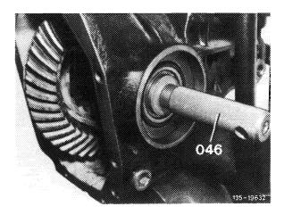
16 Move differential into position shown and take out of rear axle housing.
