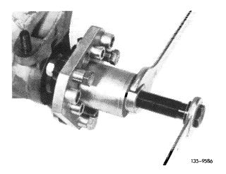
21 Force drive pinion out of rear axle housing by means of a conventional puller.
