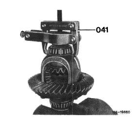
18 Unscrew ring gear from differential housing and carefully force off in relation to housing.
