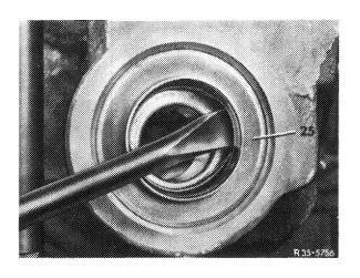
23 Screw installer and remover (038) to rear axle housing and pull inner tapered roller bearing outer race (46) out of housing by means of pulling member (038a).
