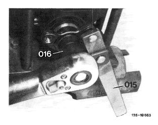
20 If required, pull universal flange from drive pinion by means of puller.
