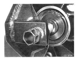
10 Preload (spread) rear axle housing to 0.20 mm by screwing-in threaded spindle of spreading device.
