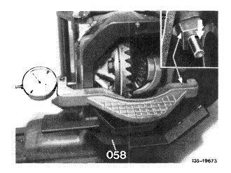
9 Turn one face of thrust piece toward opening of locking ring and screw-in threaded spindle manually up to bearing outer race.
