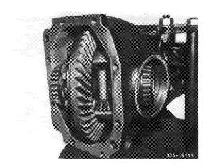
17 Pull both tapered roller bearings from differential housing by means of puller (041) and mark to prevent mixups during reinstallation.
