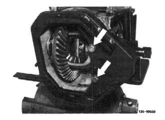
8 Place spread measuring instrument on spreading device (058) and adjust dial gauge to 0 at 3 mm preload.
