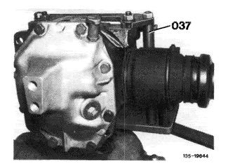
3 Unscrew end cover (57) from rear axle housing.
