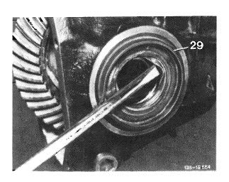
7 Attach spreading device to rear axle housing and tighten hex. screws to 40 Nm (arrows).
