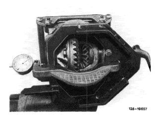
12 Remove righthand locking ring from rear axle housing by means of pliers and mark.
