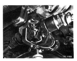
11 Unscrew rear rubber bearing on frame floor.
