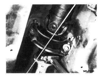
8 Unflange propeller shaft from rear axle and push forward out of concentric alignment.
