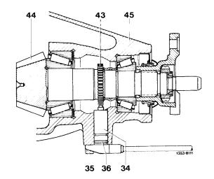
b Insert rpm sensor (34) into rear axle housing (45), making sure that the O-ring is not damaged.
