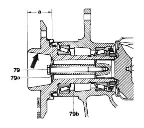
22 Lift rear axle center piece up to frame floor and attach rubber bearing to frame floor. Tightening torque of hex bolts 25 Nm. Tightening torque of self-locking hex bolts 30 Nm.
