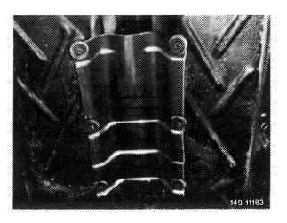
7 Loosen lock nut and unscrew propeller shaft intermediate bearing on frame floor.
