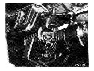
21a Tighten hex. screw for fastening rear axle shaft to rear axle shaft flange on 1st version (M 12 item 79) to 95 Nm.
