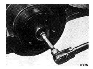
4 If required, force rear axle shaft out of rear axle shaft flange by means of assembly fixture.
