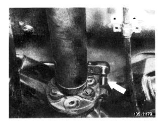
14 Lower rear axle center piece and remove together with rear axle shafts.
