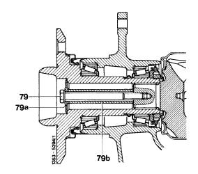
Note: Starting September 1979 the inner contour (arrow) of rear axle shaft flange has been changed and the contact surface of the tensioning disc has been displaced further inwards by 5 mm. To guarantee the correct coordination of hex. screw and spacing sleeve, measure distance "a" on rear axle flange from face to contact surface of clamping disc by means of a depth gauge and take the lengths for spacing sleeve and hex. screw from table.
