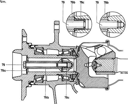
79 Hex bolt 79a Clamping disc 79b Spacing sleeve 79c Threaded bushing
