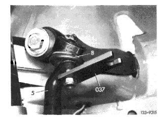
5 Steering knuckle8 Guide joint037 Spacing plate
