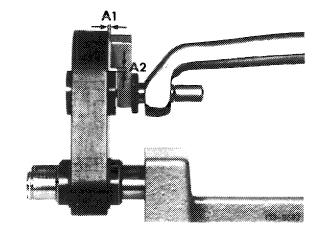
Permissible distortion of steering knuckle in direction of camber (A)
