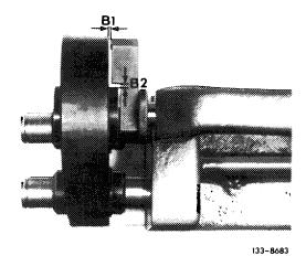
Permissible distortion of steering knuckle in direction of caster (B)  $\label{eq:caster}$
