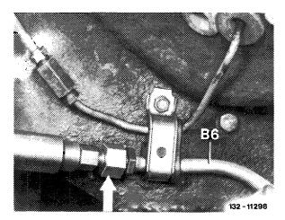
B6 Pressure line pressure reservoir-tube shock
