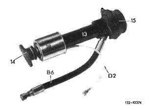
7 Insert tube shock, mount upper and lower suspension.
