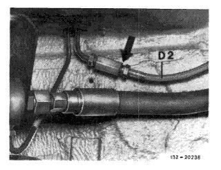
Connection leak oil hose - leak oil line D2 Return line for leak oil of tube shocks 4 Loosen upper suspension of tube shock.
