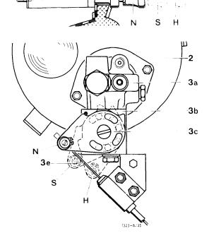
Note: To stabilize pressure in system, filling several times up to cut-out pressure is required in most cases. For this purpose, move adjusting switch for a short moment into position "M" = assembly after stopping engine and repeat filling procedure each time according to item 6.
