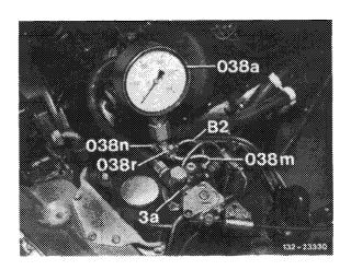
9 Check oil level in reservoir and correct, if required. Check line connections for leaks (32-600).
