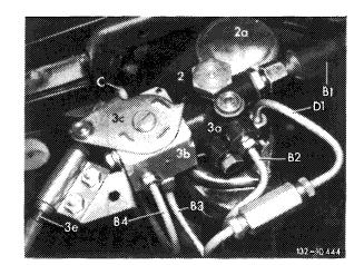
3 Connect pressure gauge (038a) with distributor (038r), pressure test line (038m) and vent screw (038n) between pressure regulator (3a) and pressure line (B2).
