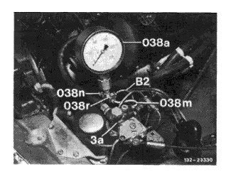
Connection of pressure tester models 126.033, 126.037
