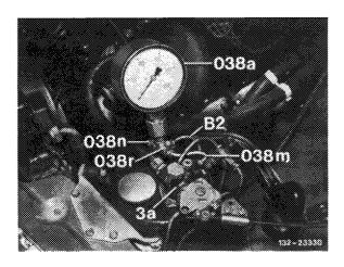
4 Disconnect pressure line (B4) adjusting switch—level controller and control pressure line (C) on adjusting switch (3b) and close with vent screw (038n) at adjusting switch.
