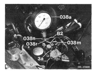
7 Check oil level in supply tank and correct. Check line connections for leaks (32-600).
