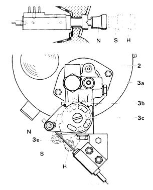
8 If no pressure is established in pressure regulator (3a), contamination in filter of throttle screw may be the cause.
