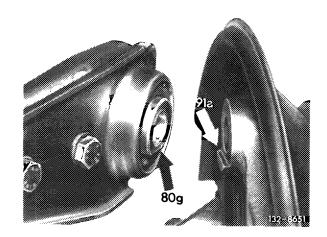
9 Connect torsion bar support to wheel carrier
