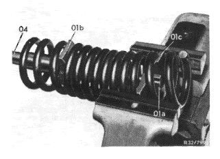
01a Tensioning screw 01b Upper tensioning plate O1c Lower tensioning plate O4 Socket
