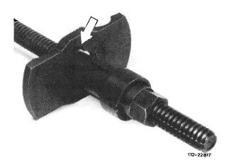
5 Tension front spring, while lifting lower control arm by means of a vehicle jack to facilitate tensioning.
