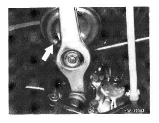
8 Tension front spring at 9, but at least 8 coils. Apply tensioning plates offset by  $90^{\circ}$
