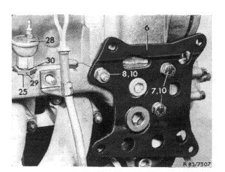
2 Remove plug with the 17 mm screwdriver socket.
