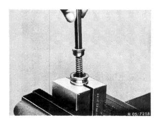
19 Guide chain tensioner into chain tensioner hole in cylinder head with an internal socket wrench.
