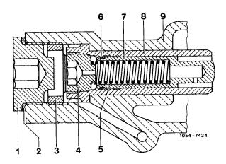
3 Loosen ball locating ring (oil jet) by about 2 turns with a socket wrench.
