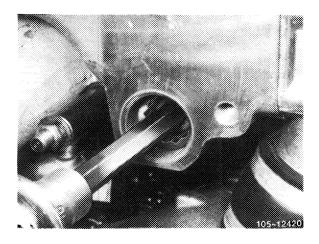
4 Remove threaded ring with a 19 mm screwdriver socket.
