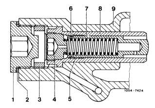
24 Install threaded ring (3) and torque to 50 Nm.
