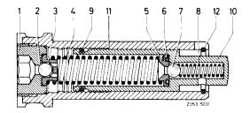
The pressure pin cannot be pressed back beyond the saw tooth type catch in assembly position,,A".
