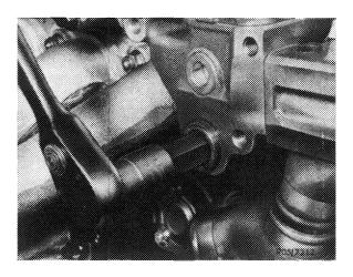
5 Pull out chain tensioner with a 10 mm socket wrench.
